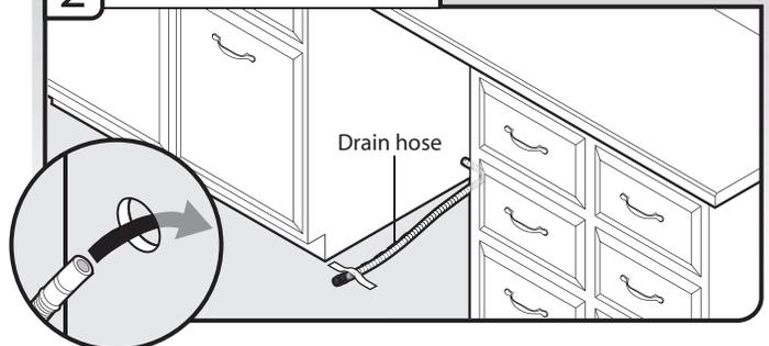
Route drain hose as shown through hole in cabinet to the front center of opening where drain connection will be made. Tape drain hose to the floor in area shown. This will keep the drain hose from moving when dishwasher is moved into cabinet opening.
